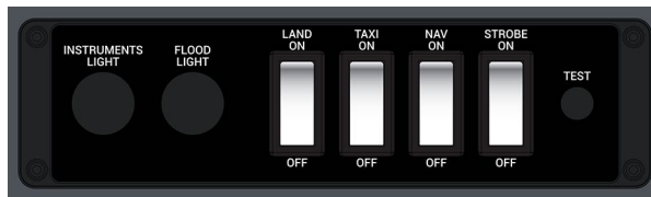
Figure 6.63: Light switches on the dashboard
