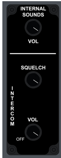
Figure 6.44: Intercom Control Panel
