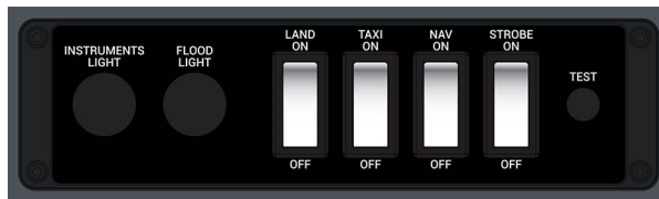
Figure 6.58: Light switches on the dashboard
