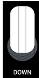
Figure 6.16: Landing Gear Control
