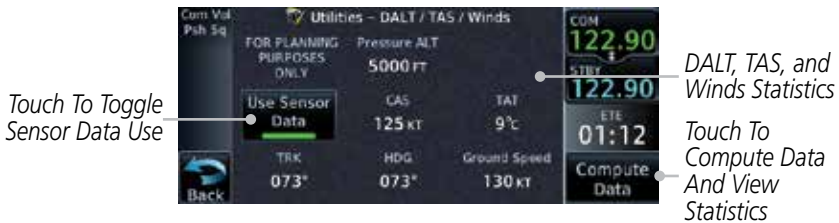
Figure 14-37 Utility DALT/TAS/Winds Page Using Sensor Data and Pressure Altitude
