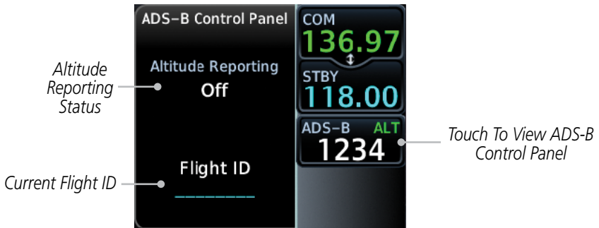
Figure 2-13 ADS-B Control Panel
