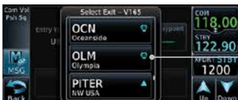
Figure 4-21 Select an Exit Waypoint for the Airway
