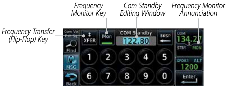
Figure 3-26 Com Frequency Monitoring
