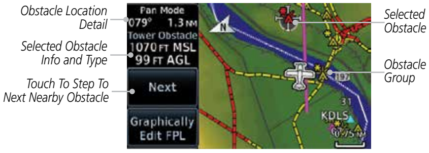
Figure 8-21 Point Obstacle Detail
