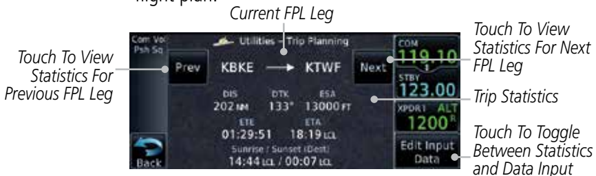
Figure 14-26 Utility Trip Planning Page Computed Data View Of Next Waypoint (Flight Plan Mode)
