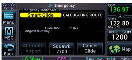
Dual GTN Xi configuration with dedicated map display on GTN 750Xi (GTN 1) and Emergency page on GTN 650Xi (GTN 2).
